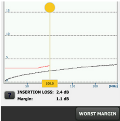
Figure 1. Measured Insertion Loss and limit for 100 foot Type 734 cable.
