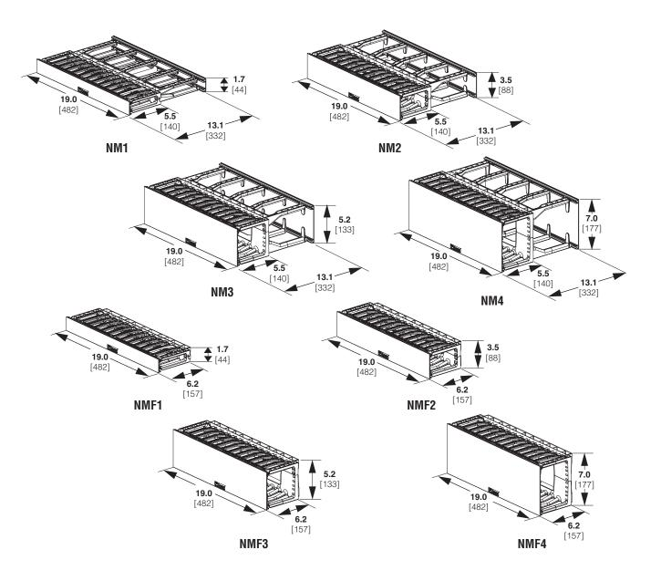
Dimensions are in inches. (Dimensions in parenthesis are metric).
